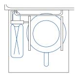
If, for any reason, the dishes do not fit properly into the holder, do not load the rinsing chamber with the dishes in question. Urine bottles are pushed (with the opening to the front) through the retaining ring on the left-hand side as far as the stop. Bedpans and commode buckets are pushed into the holder with the opening facing upwards. The lid of the bedpan
